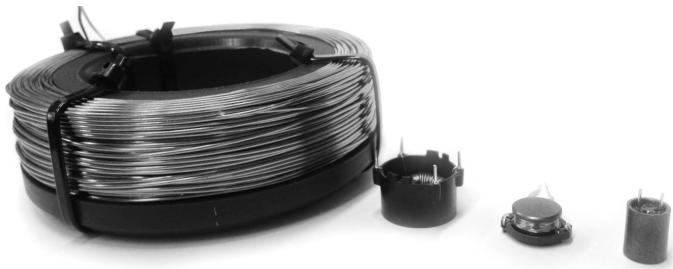
Figure 6.12: The coils used in the experiment. From left to right: 6.7 mH, 10 mH, 1 mH and 100 mH.
