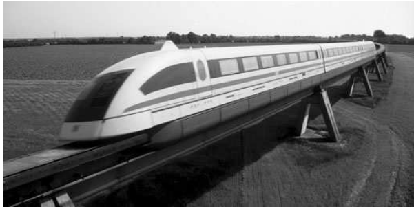
Figure 1.3: The German MagLev, a big linear motor and generator.
